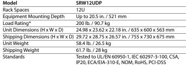
\* The load rating includes the combined weight of the unit and installed equipment. The unit must be mounted to a stable surface with user-supplied anchors capable of bearing the full load.
